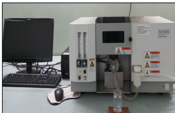
Figure 3.7 Atomic Absorption Spectrophotometer (Shimadzu AA 6200)
