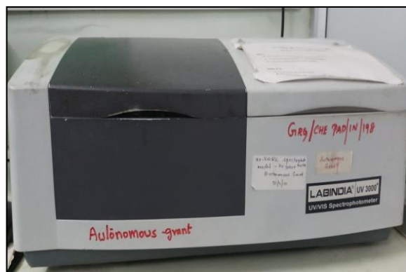
Figure 3.6 UV-Visible Spectrophotometer (Lab India UV 3000 +)
