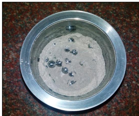
Figure 8.2 Jar with Sorbent and Tungsten Carbide Balls
