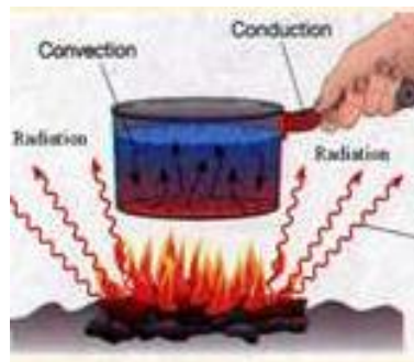
Fig 1.15 Example for conduction, convection and radiation – Heating the liquid in a pan
