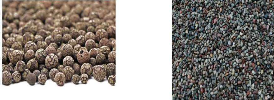
Fig 1.6 Granular porous materials used in the construction industry, Liapo ® spheres and crushed limestone
