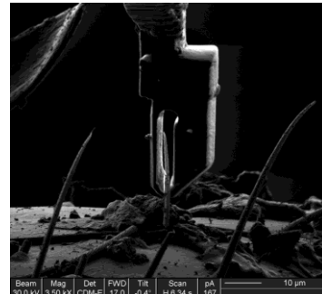
Fig.4. Capture of a biomicro object, a sensillum of Culex pipiens , by T 2 NiCu composite nanotweezers with SME.
