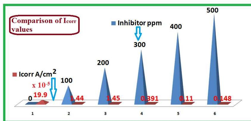
**Figure 5.** Comparison of  $I_{corr}$  values of MS immersed in various test solutions.
