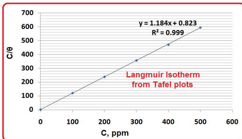
Figure 11. Langmuir's adsorption isotherm (from the polarization study).
