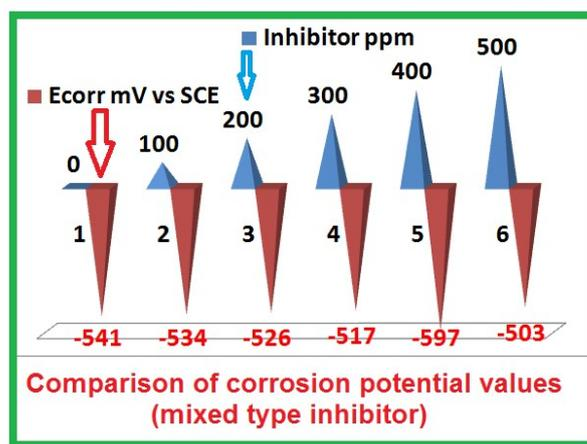
Figure 6. Comparison of  $E_{\text{corr}}$  values of MS immersed in various test solutions.
