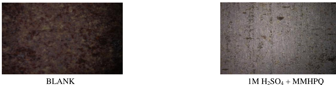
Figure 8. Optical Microscope images of mild steel surface without and with the addition of MMHPQ
