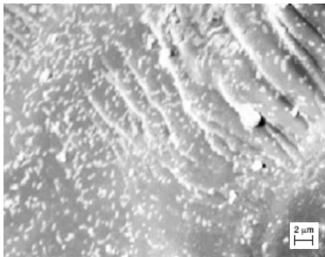
Figure 1. SEM micrograph of the surface of sago waste carbon, Magnification- 2500x
