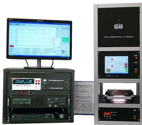
Figure 2.3 Solar simulator set up for I-V measurements
