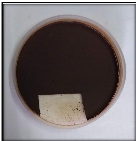
Figure 6.1: Biopolymer electrolyte membrane - SGMC
