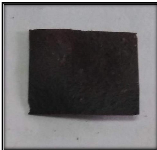
Figure 6.3: Biopolymer electrolyte membrane - SGAF
