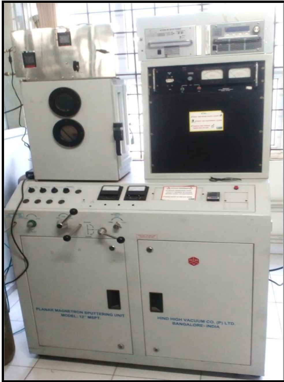
Figure: 5.3. Photograph of DC magnetron sputtering unit for fabricating IDA electrodes
