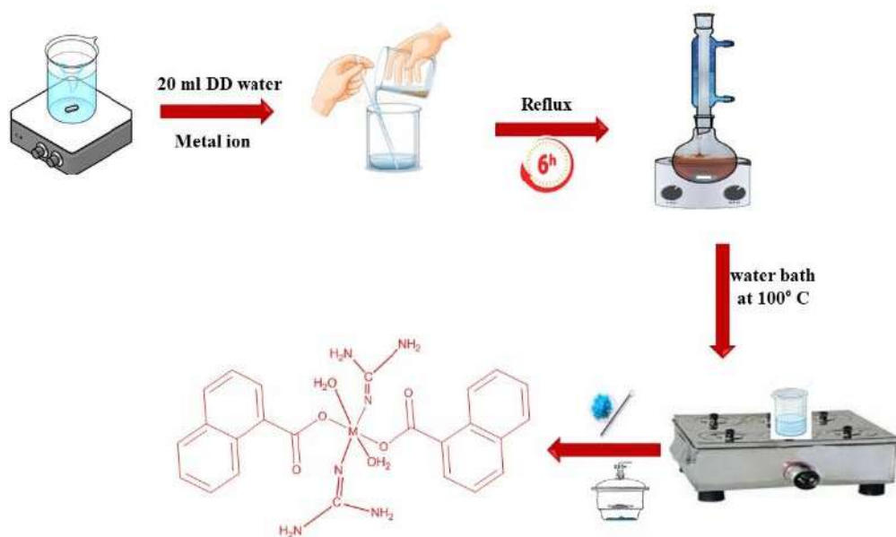
Figure 8.1 Synthesis of metal complexes
