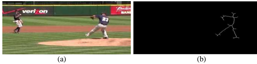
Figure. 4 (a) Sample input video block and (b) Outcomes of joint and trajectory coordinate extraction
